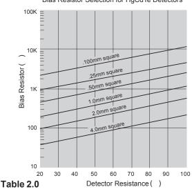
3. The bias resistor ( $R_B$ ) is selected to balance the bridge network and must be selected to provide all of the current to the detector. The value of  $R_B$  can be calculated using the following formula or Table 2.0.
